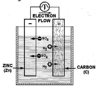
3. The result is a charge separation or a potential difference between the two terminals (electrodes).
