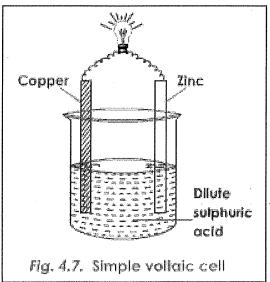
2. The zinc in this case acquires negative charge while the copper acquires positive charge.
