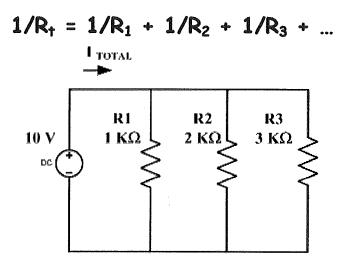
$$1/R_{t} = 1/R_{1} + 1/R_{2} + 1/R_{3}$$
