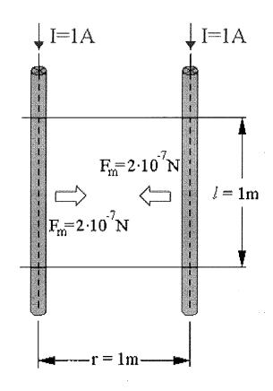
$$F_1 = \underline{\mu_0} \, \underline{I_2} \, \underline{I_1} \underline{I_1}$$
