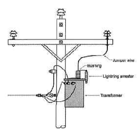
1. A transformer is a device that increases or decreases AC voltage. It has three basic parts: a primary coil, a secondary coil, and an iron core.
