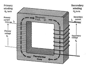
2. An alternating current goes into the primary coil producing a magnetic flux in the iron core. The iron core transfers the magnetic flux to the secondary coil. The secondary coil produces an induced EMF to counter the introduction of the magnetic flux in the iron core.
