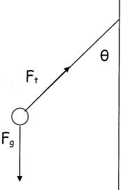
2. The force of tension acts along the rope while the weight acts straight down. The force of tension provides the center seeking force and is the horizontal component of the  $F_{t}$ .
