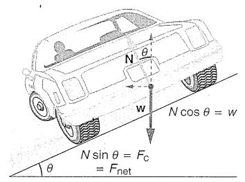
For a car going around a curve with radius r travelling at speed v, determine the formula for the angle at which a road should be banked so that no friction is required. What is the angle for a curve of radius 50m at a designated speed of 50km/h?
