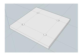
4 Erase construction lines as necessary. Voila! You have your through-holes!
