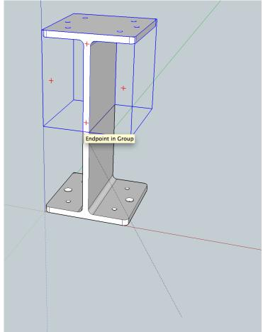
8. Once this is done, select a half, right click, select 'Explode'. Repeat for the other half and erase the 4 dividing lines. This effectively joins the two parts into one.
