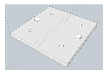
2. Extrude the rectangle up by 70mm to create the "T" flange and erase any necessary guidelines.
