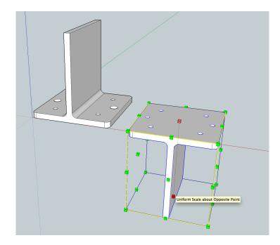
7. Now we can use the move tool to move the reflected part onto the original part. Using the move tool, click a corner on the surface of the "T" to be butt against the corresponding location on the original part.
