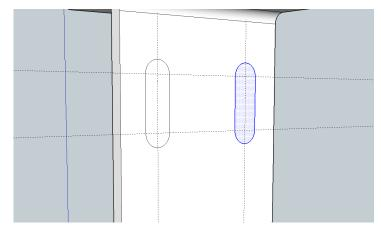
5. Then right after clicking the mouse to release the object, type in "/2." What this does is it creates two copies of the object you just duplicated and it positions them evenly spaced across the distance the object was moved.
