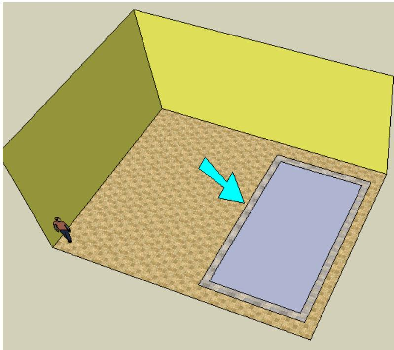
5. Pull up the pool walls, and pull up the floor to make the water line. When you use **Push/Pull** for this, keep the Ctrl / Option key pressed. This means that the bedroom floor will stay intact, instead of being “sucked up” with the pool objects. (Try it first without the Ctrl / Option key to see the difference). If the water doesn’t seem deep enough, pull the bedroom floor down (*without* the Ctrl / Option key).
