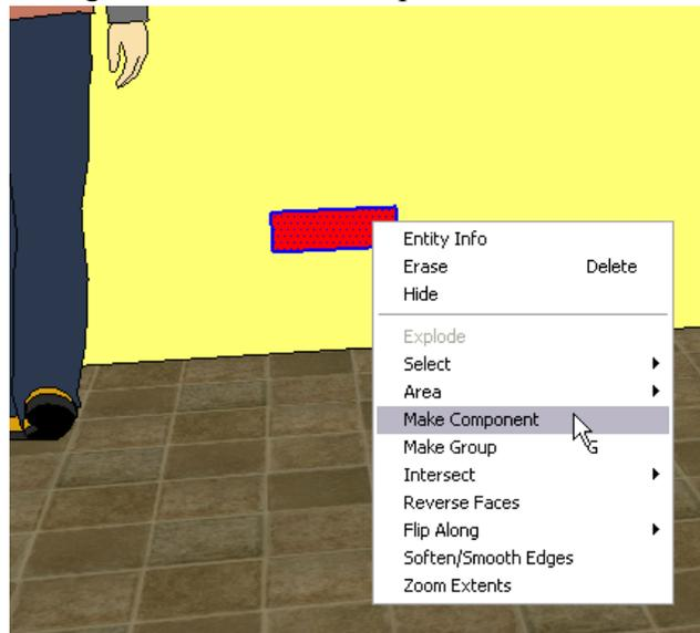
12. Edit the component, and pull the step out about 1200mm.
