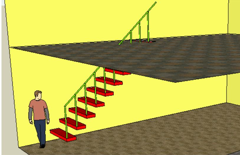
20. We want to go up the steps without hitting our heads on the floor above, so cut a hole out of the loft floor.
