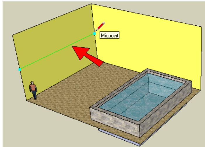
8. Make the floor long enough to hang a little over the pool (Line 2). When you make Line 3, start drawing in the direction you want the line to go (green, in my example). Press Shift to “lock” the direction, and click the first point of Line 1. This sets the exact length of Line 3.
