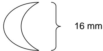
$$\begin{aligned} \text{DM} &= \frac{\text{Drawing Size}}{\text{Actual Size}} \\ &= \frac{16 \text{ mm}}{0.8 \text{ mm}} \\ &= 20 \text{ x} \end{aligned}$$
