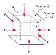
Example: If a block of 1  $\text{m}^3$  concrete block is submerged in water to a depth that has a pressure of 1.1065 x 10 $^6$  Pa (Pascals), then what will be the change in volume of the block? Surface pressure is 101325 Pa.
