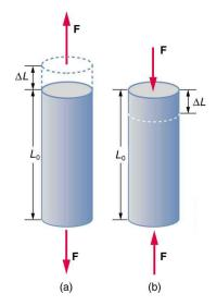
12. There are three types of stress, the above 2 and shear stress. With shear stress the object has equal and opposite forces acting on opposite faces.
