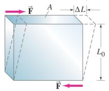
13. The object dimensions do not significantly change but the shape of the object does change. An equation similar to the equation in number 6 can be stated for shear stress.
