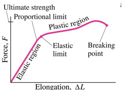
3. The above relationship is said to be linear up to the proportional limit. Beyond the proportional limit is the elastic limit which is the point that if the force is removed then the material will still return to its original length.
