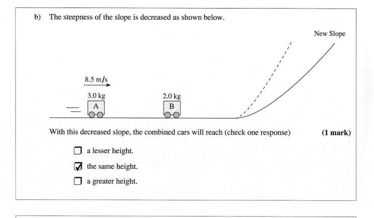
The steepness of the slope does not matter. All of the cars kinetic energy will be transferred to gravitational potential energy. Since the original kinetic energy of the cars has not changed, they must have the same potential. Therefore, they go to the same vertical height.
