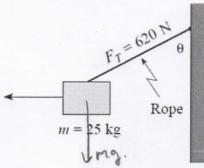
To what maximum angle,  $\theta$ , can the block be pulled without the rope breaking?
