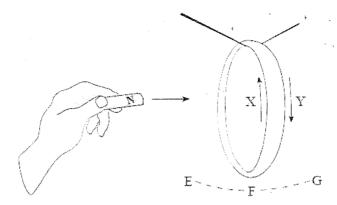
Determine the direction in which current will flow in the ring and the direction in which the ring will move.
