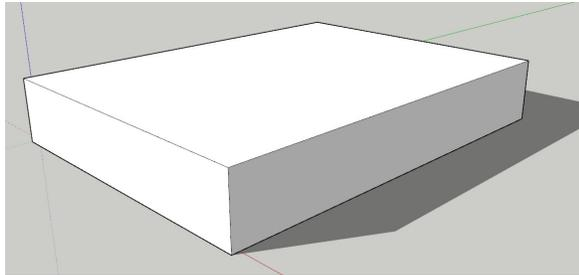
2) From the bottom front corner, draw a line up along the front edge 150 mm long.
