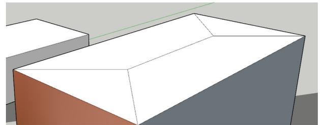
6. Use the Move tool to lift the middle line up on the Blue (Z) axis
