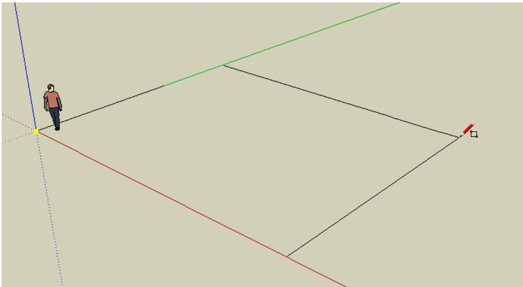
2. Many of SketchUp's tools can use exact numbers. While you're using the **Rectangle** tool, look at the **Dimensions** box below the SketchUp window. You'll see the length and width of the rectangle change while you move the mouse. Make this rectangle about 10 metres wide and 14 metres long. (If you want the numbers to be exact, you can type them in and press Enter. Be sure to include the apostrophe foot symbol, and separate the two numbers with a comma.)
