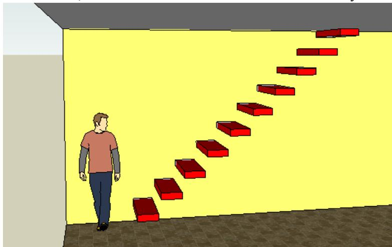
15. Components are also great for making railings. Edit any step, and draw a vertical (blue) line in the lower corner, about 1m (1000mm) high.
