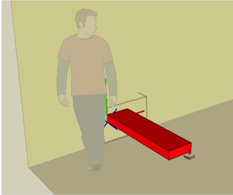
13. Close the component, and then make one copy at the top of the loft floor.
