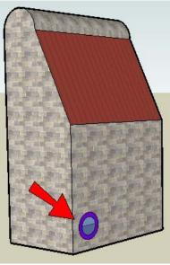
This window needs to be made into a component since we'll use it repeatedly. As a component, the window will be much easier to select - it acts as one object. (Components also have the advantage of being "unsticky" - it's much easier to move and rotate components without affecting objects they touch.)
