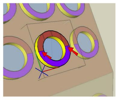
19. To make the cover, use **Push/Pull** but press the Ctrl / Option key. This way you'll be adding a new part, instead of pulling out an existing face.
