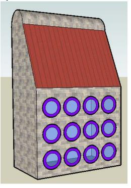
9. Copy some or all of the windows up to the sloped face. Even though the original windows make cutouts on the vertical wall, the new windows also cut the sloped wall.
