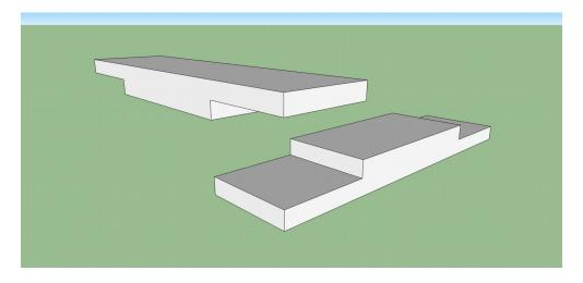
Glue together the frame pieces (make sure to check for 90 degree corners!) When dry (the next day), sand flat if necessary.
