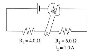
When a wrench that has a small resistance is dropped on the circuit as shown, the current through R<sub>2</sub> is reduced to 1.0 A. What is the current flowing through the wrench? (Assume the supply voltage remains constant.)
