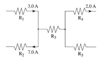
What are the magnitude and direction of the current passing through resistor R<sub>5</sub>?
