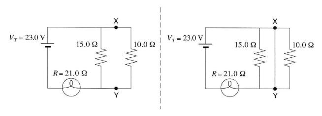
What is the current through the light bulb and what happens to the brightness of the bulb when the wire is connected?
