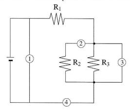
In which locations should an ammeter and voltmeter be connected to correctly measure the current through  $\,R_2\,$  and the voltage drop across  $\,R_2\,$ ?
