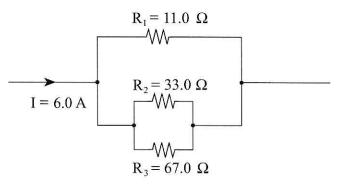
What is the current through resistor  $R_1$ ?
