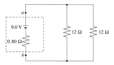
$$\frac{1}{R \text{ parallel}} = \frac{1}{12} + \frac{1}{12}, R \text{ parallel} = 6.0 \Omega$$
