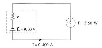
a) If a current of 0.400 A leaves the battery, what is the internal resistance, r, of the battery?
