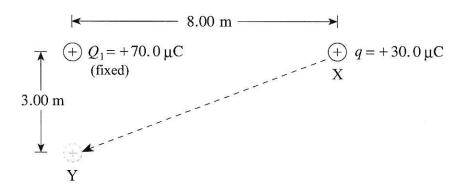
How much work is done on the 30.0  $\mu$ C charge?  $(1 \mu C = 1 \times 10^{-6} \text{ C})$
