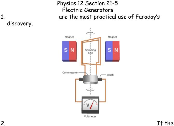
above Coil is rotated by some external force then the magnetic flux (BAcos (changes))
